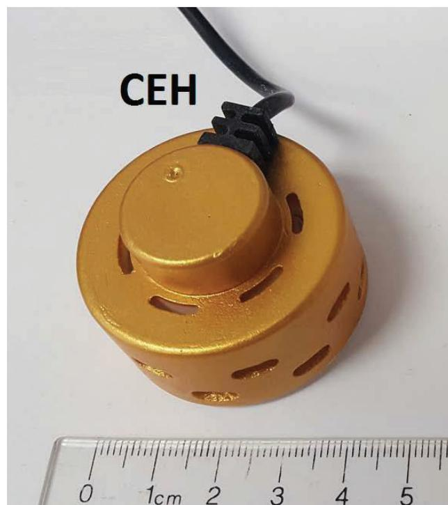
charcoal (Three Kings Holland, 40 mm diameter) heating system to heat the tobacco in the waterpipe smoking sessions. The commercial waterpipe electric heater was powered by the manufacturer's power supply (stated as 13 V DC and 3.5 A current). However, based on internal measurements, the voltage measured 14 V DC with 2.7  $\Omega$  resistance, resulting in approximately a 5.2 A current.
